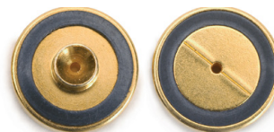
Figure 1: Vespel rings on both the top and bottom surfaces simplify installation by reducing the torque requirement and eliminating the need for a washer.
